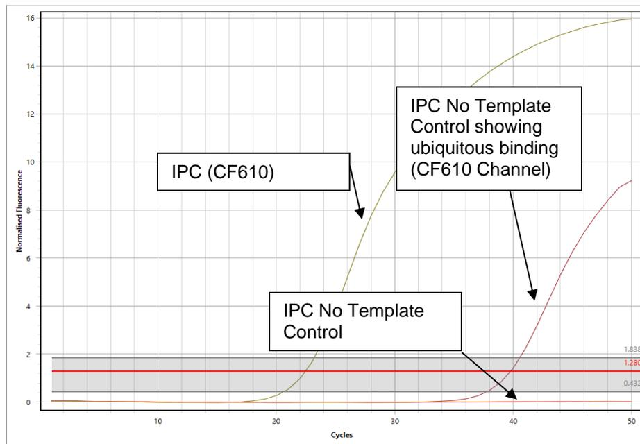
*Figure 3: Ubiquitous Binding of No Template Control in the IPC CF610 Channel*
